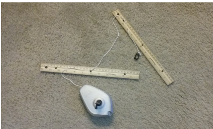
FIGURE 2. Equipment needed to check crown.
