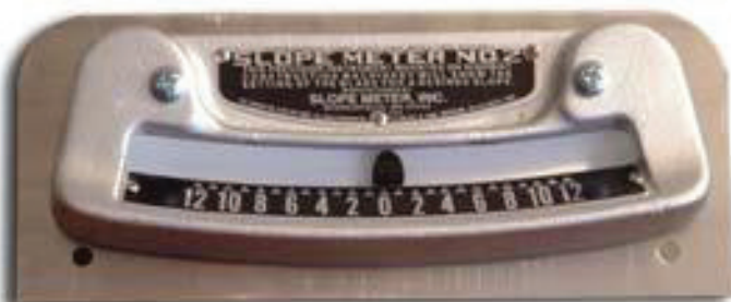
FIGURE 3. Slope meter should be marked at the desired cross slope, usually at the 4.
